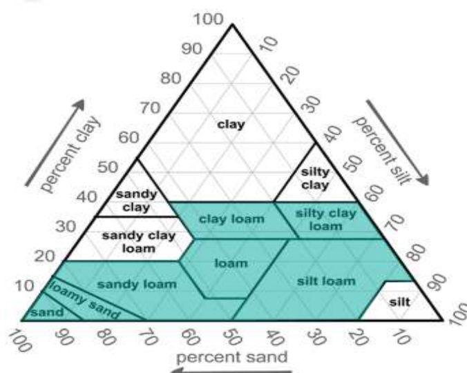
Figure 14: Soil Textures defined by Salinity Calibration equations (shaded).
