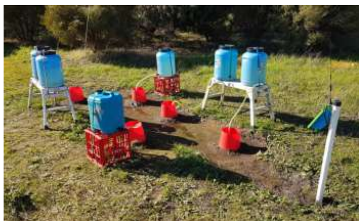
Figure 2: Field setup of Benchmarking site showing 6 different salinity treatments. Data was collected using a Bluetooth Hub Unit via aerial connection to the web.
